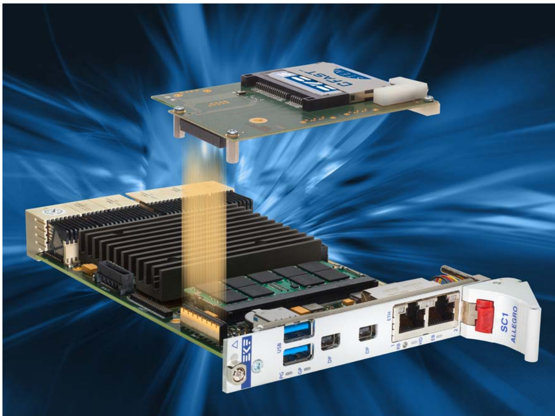
SC1-ALLEGRO with C41-CFAST Low Profile Storage Module
