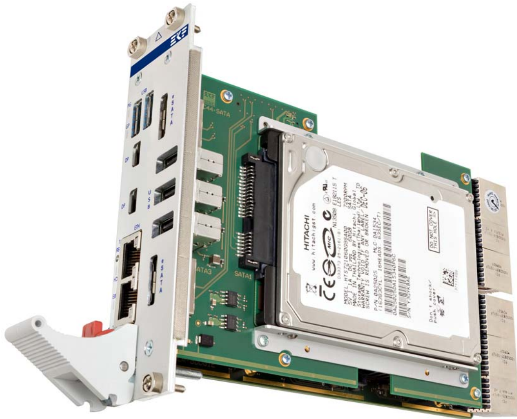
SC1-ALLEGRO with C44-SATA Assembly (8HP Front Panel)
