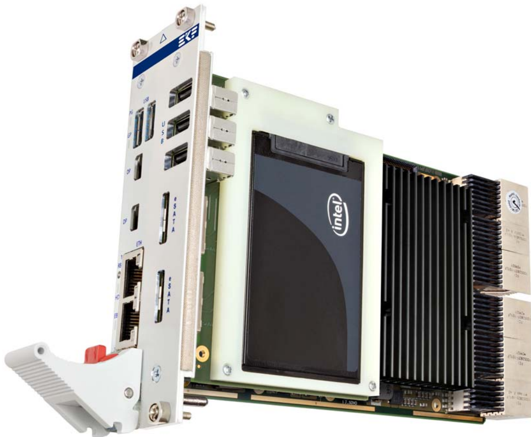
SC1-ALLEGRO with C45-SATA Assembly (8HP Front Panel)
