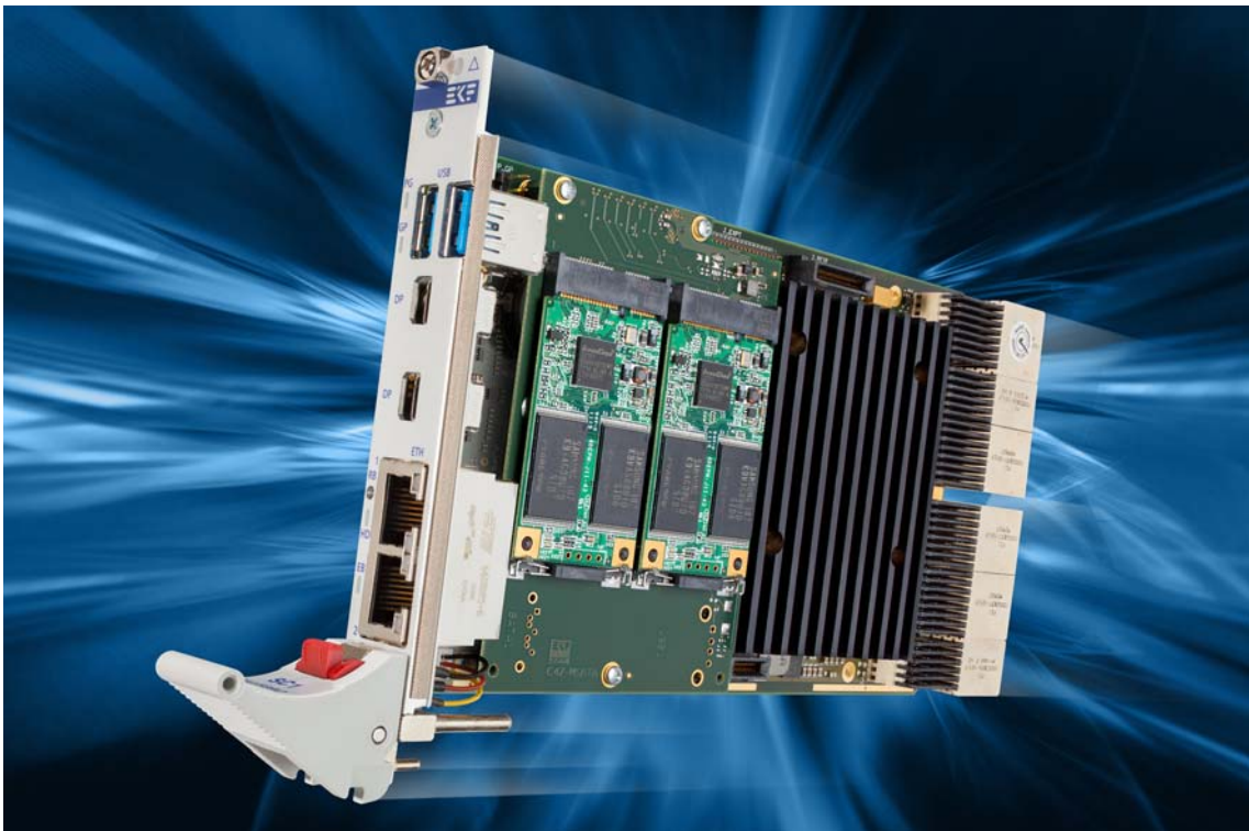
4HP Front Panel Width with C47-MSATA
